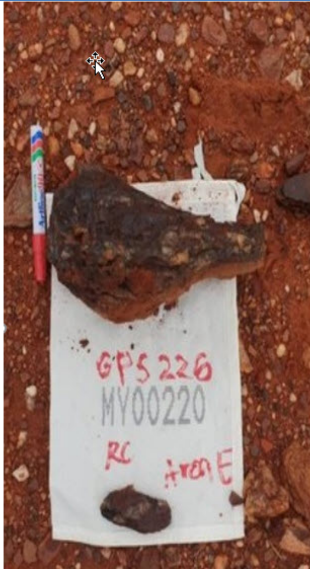
Figure 14: Rock chip sample of sheared metamorphosed mafic/BIF contact with Quartz breccia and weathered ex sulphide carbonate
