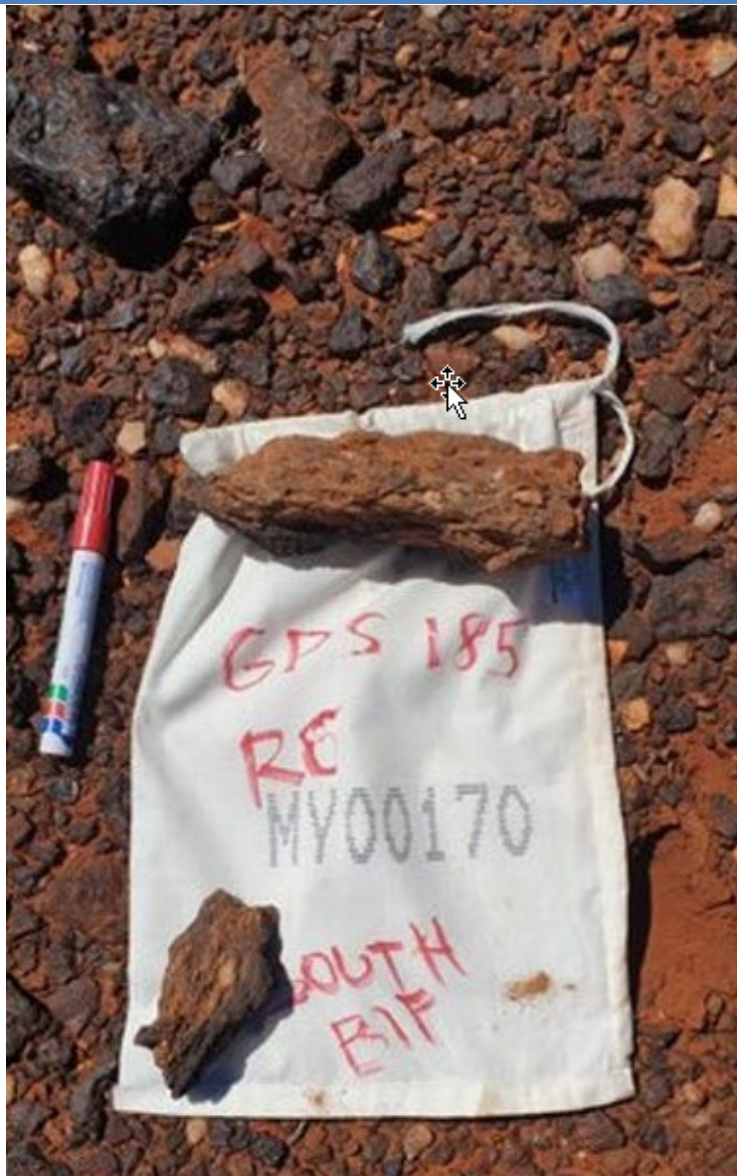
Figure 11: GPS 185 Sample location. Strongly sheared altered mafic rock associated with BIF
