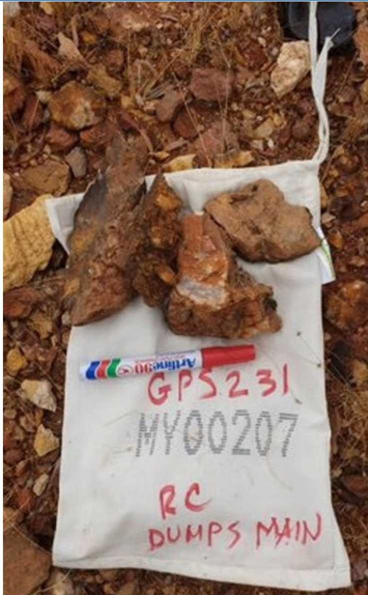
Figure 13: GPS Sample location 231. Sheared mafic/felsic rock sample with strongly brecciated Quartz veining
