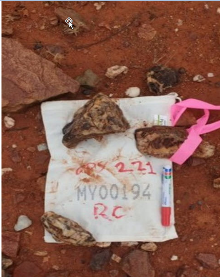
Figure 12: GPS 221 Sample Location. Strongly sheared altered metamorphose mafic/Quartz veining, hematized and excarbonate/sulphides alteration
