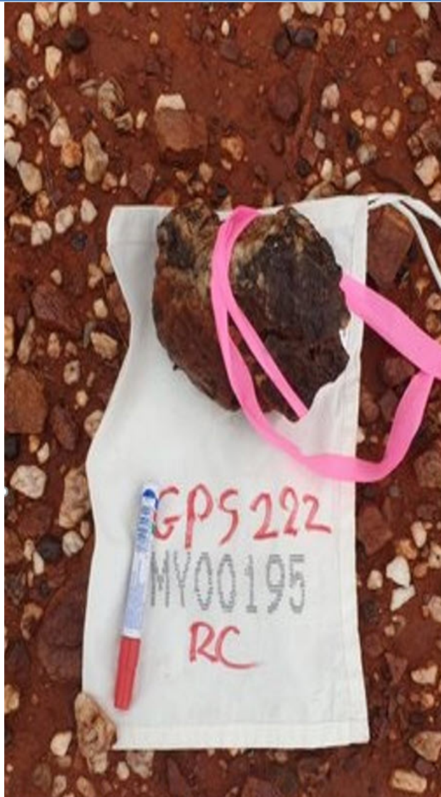
Figure 15: Massive BIF sample associated with Quartz breccia and ex carbonate /sulphide
