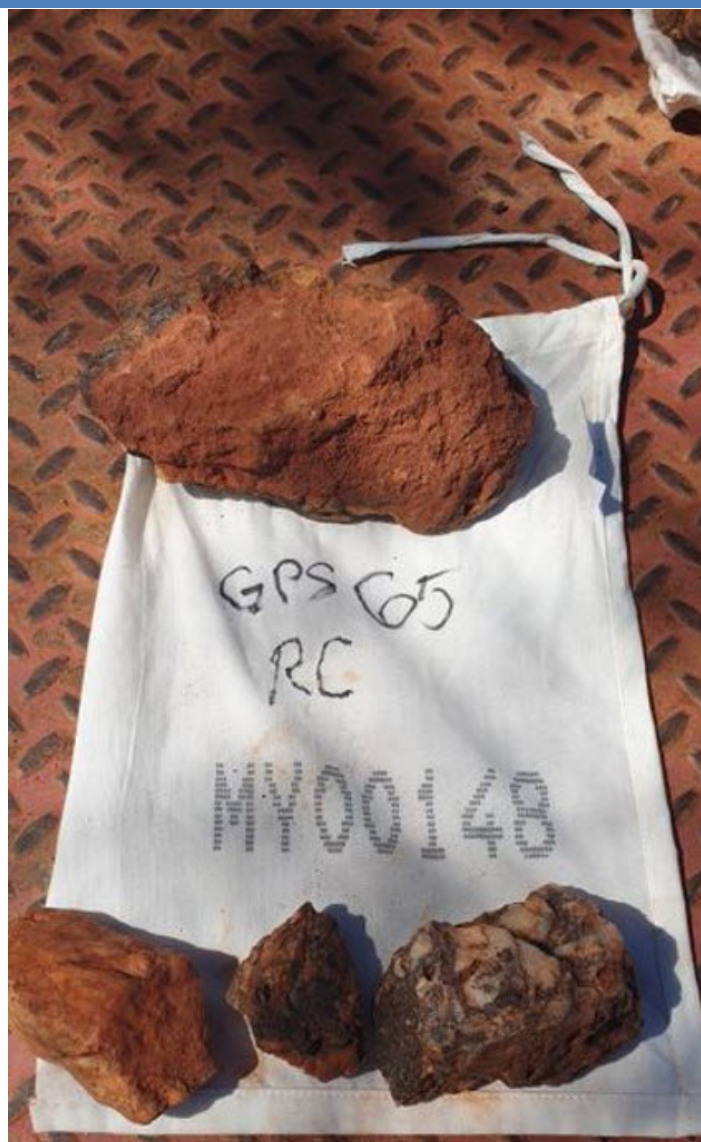
Figure 16: Weathered strongly silicified mafic rock associated with Brecciated Quartz
